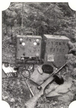
Fig. 4: The VRKS v.h.f. manpack set, with a few self-defence items (see text).
