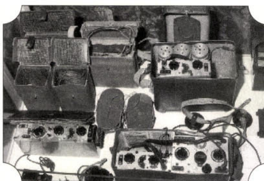
Fig. 5: The VRHAG collection of clandestine transceivers, used by Finnish guerrillas (see text).
