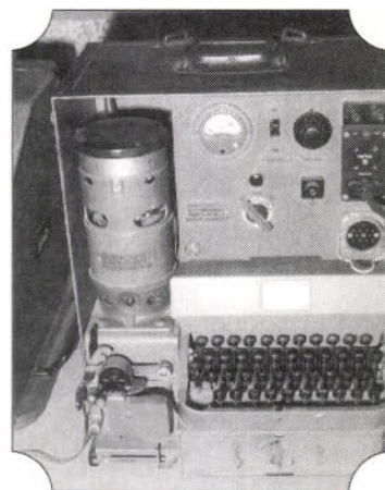
Fig. 2: The German Hellschreiber machine, showing the keyboard. The motor on the left forms part of the image scanning system.
